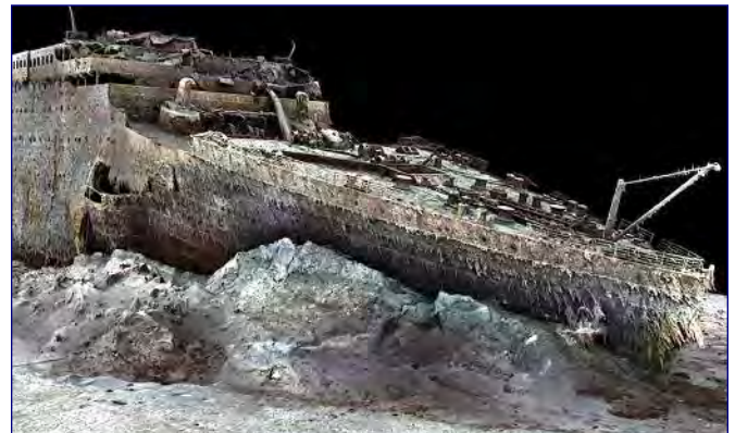
Below: The image shows how the bow was driven into the seabed.
