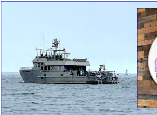
The Barracuda, above, is a 74-ft x 27.5-ft aluminum hydrofoil catamaran obtained by CDFW in 2024.
